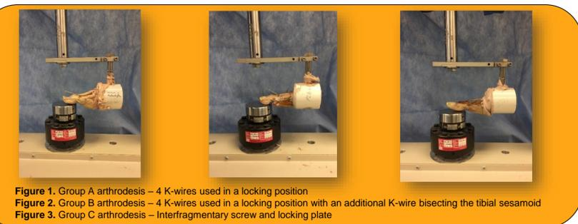
Figure 1. Group A arthrodesis – 4 K-wires used in a locking position
