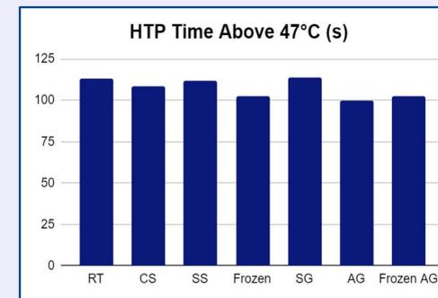
Figure 4: Mean time above 47°C with HTP method
