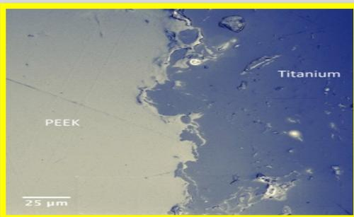
Figure 5 – Cross-sectional SEM of the Ti-PEEK interface.
