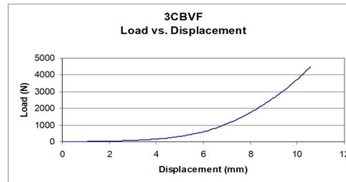
Figure 3. Load versus displacement curve for specimen 3CBVF. There is no evidence of a significant decrease in the slope of the curve or a sudden drop in load.
