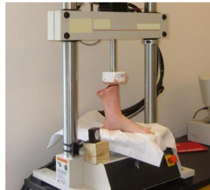
Figure 2. Image of foot specimen loaded into biomechanical test system.
